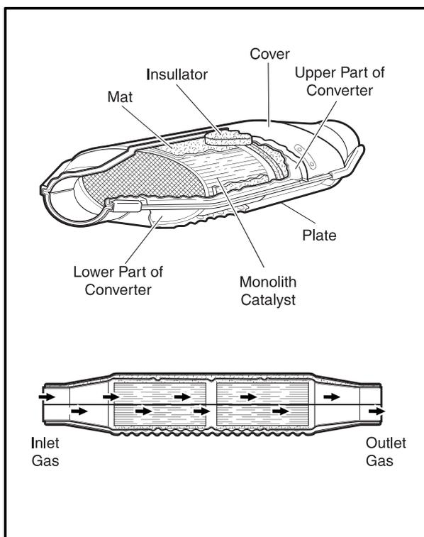
The Catalytic converter of monolith type consists of 2 walled metal bodies which is made of Cordierite. The principal element of converter consists of the materials like Alumina or oxidized Serume in order to apply to Ceramic Monolith. Washer coat operates first, and catalytic metal elements (Pt, Pd, Rh) operates to washer coat next.
