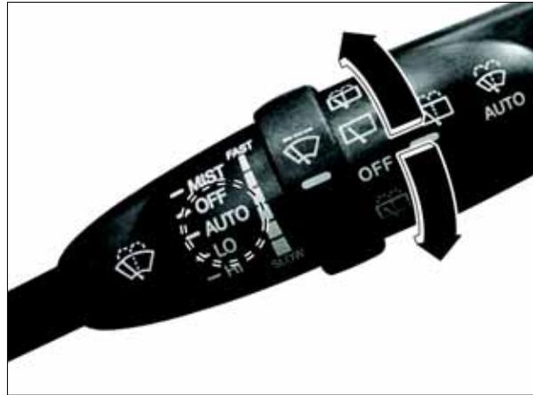
**AUTO:** Wiper operates automatically by rain sensor
