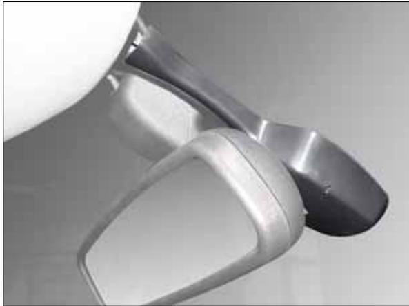
A sensor that emits infrared rays through LED and then detects the amount of rain drops by receiving reflected rays against sensing section (rain sensor mounting section on the windshield) with photodiode. The auto light sensor is Integrated into the rain sensor (refer to the below picture).
